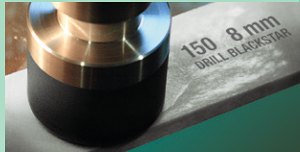
Sharpening of a monobloc drill with a WENDT™ sharpening stone
