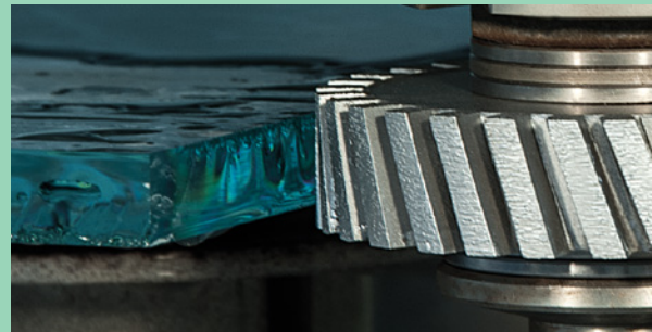
Machining of glass with segmented grinding wheel Silver
