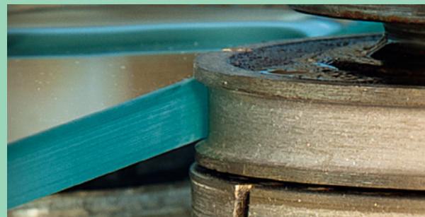
Edge grinding with STAR TRACK Flat & Arris wheel
